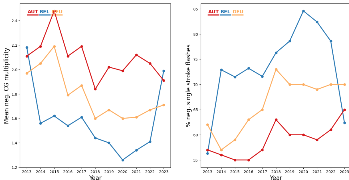
Figure 5 Annual distribution of (a) the mean multiplicity in negative flashes and (b) percentage of single stroke flashes in Austria (AUT), Belgium (BEL) and Germany (DEU).
