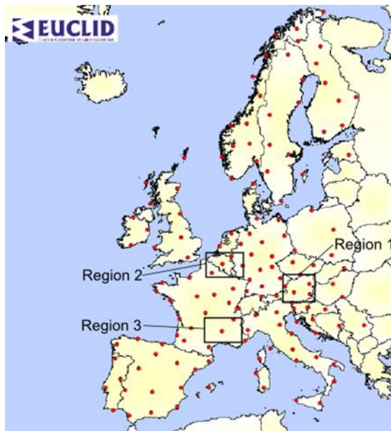
Fig. 1: EUCLID network configuration for 2012. Sensor locations are shown as red dots.
