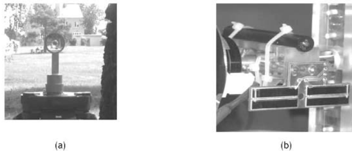
Fig. 11. (a) The corner cube reflector used as a target, (b) The photocells receiving the light reflected from the reflector.
